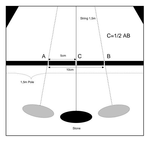
Whenever you pivot the one foot of the A frame up or down slope, the string will move one way or the other across the crossbar. When your string comes to rest at the calibration or level mark (C), this is when the two feet are on level ground.
